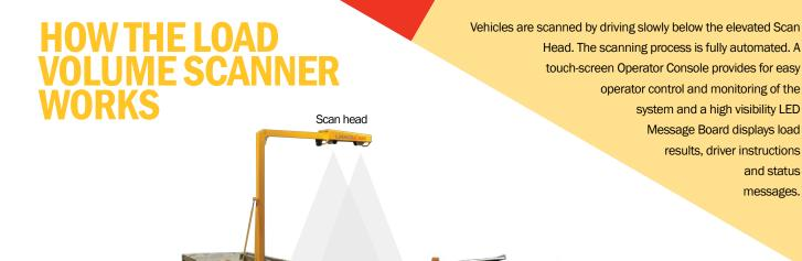
In standard operation, vehicles are scanned empty and recorded in the system database. On subsequent visits the loaded vehicle is scanned and the load volume computed by comparing load scans against database records. Trucks
