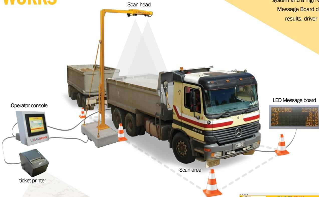
In standard operation, vehicles are scanned empty and recorded in the system database. On subsequent visits the loaded vehicle is scanned and the load volume computed by comparing load scans against database records. Trucks and trailers can be identified manually, or they can be fitted with RFID tags that automatically identify the vehicle(s) when scanned.
