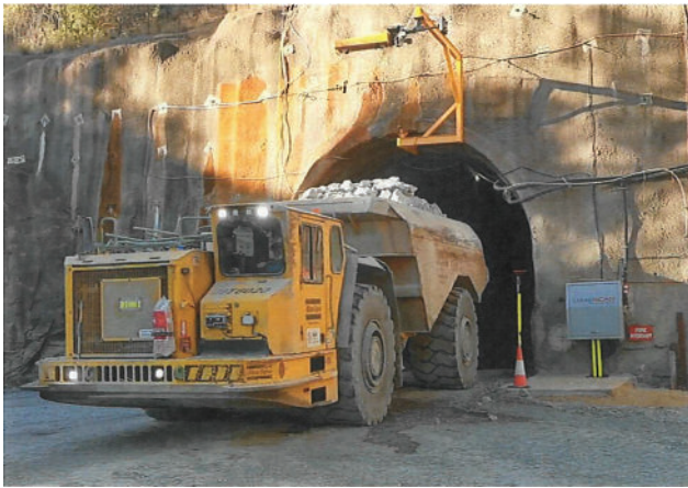
Figure 1. Photograph of loaded truck exiting the portal and portal-mounted load volume scanner
